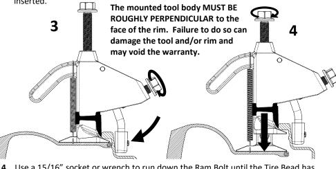
4. Use a 15/16" socket or wrench to run down the Ram Bolt until the Tire Bead has been pushed past the Bead Retainer on rim. Depending on the age of the tire and condition of the rim, the bead may partially return to the seated position. Make sure not to run the Ram Bolt past the point where the flange head contacts the tool body, which may result in stripping out the threads.
