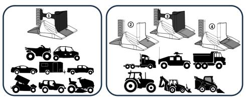
The majority of smaller wheel applications require the SHORT FOOT w/ SPACER. Large wheel applications such as Agricultural, Industrial and OTR have larger rim lips and may require one of the other tool configurations. The goal is to choose a foot length that gets close to the Bead Seat of the rim without touching it, so that it has clearance with the Bead Retainer. Using too short of a foot may miss the Bead Bundle all together and could puncture the sidewall.
