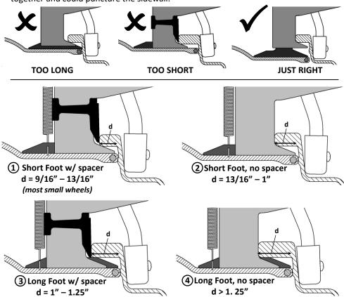
If you are unsure of your Rim Lip Depth, you can approximate it by measuring the outermost diameter of the lip of the rim, and subtracting the inside diameter of the tire (Standard Tire Diameter).
