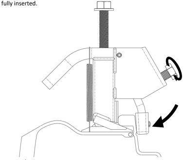
**4.** Using a 15/16" socket or wrench, run down the ram bolt until the tire bead has been pushed past the retaining lip on rim. Depending on the age of the tire and condition of the rim, the bead may partially return to the seated position. Make sure not to tighten the ram bolt past the point where the flange head contacts the tool body, which may result in stripping the threads out.
