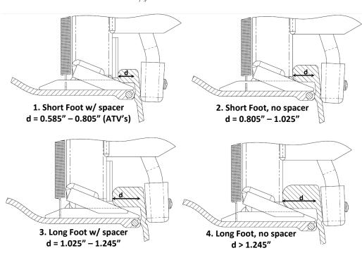
If you are unsure of your rim lip depth, you can approximate it by measuring the outermost diameter of the lip of the rim, and subtracting the inside diameter of the tire (standard tire diameter).
