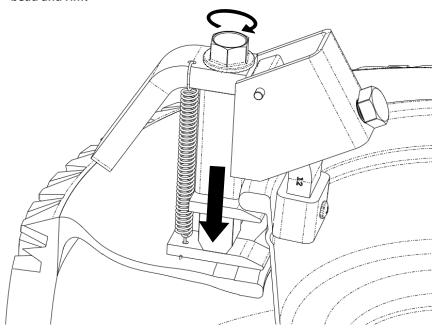
**5.5.** Loosen the ram bolt and clamp bolt. Move the BeadBuster to another location on the rim 2-3 inches from the first location. Tighten the clamp bolt and drive the ram bolt to break the bead. Repeat this process until the tire bead is completely loose from the rim.
