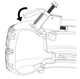
5.3. Using a 3/4" socket or wrench, tighten the clamp bolt on the BeadBuster using a small impact tool or hand wrench. Tighten the clamp bolt until the BeadBuster is vertical, and the body is touching the rim. Make sure the BeadBuster feet are fully inserted. Over-tightening the clamp will cause the tool to lean back and the ram foot to catch on the Bead Retainer of the rim! The Clamp Pad assures that the BeadBuster will not scratch your rims.
