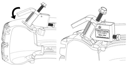
5.3. Using a 3/4" socket or wrench, tighten the clamp bolt on the BeadBuster using a small impact tool or hand wrench. Tighten the clamp bolt until the BeadBuster is vertical, and the body is touching the rim. Make sure the BeadBuster feet are fully inserted. Over-tightening the clamp will cause the tool to lean back and the ram foot to catch on the Bead Retainer of the rim! The Clamp Pad assures that the BeadBuster will not scratch your rims.
