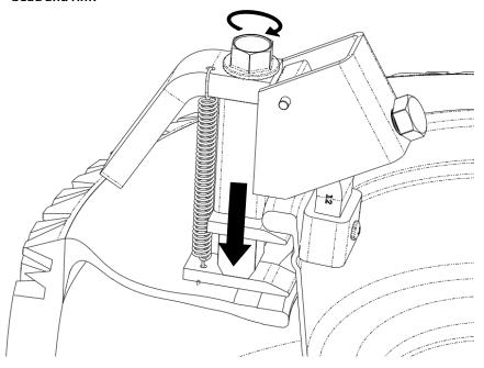
**5.5.** Loosen the ram bolt and clamp bolt. Move the BeadBuster to another location on the rim 2-3 inches from the first location. Tighten the clamp bolt and drive the ram bolt to break the bead. Repeat this process until the tire bead is completely loose from the rim.
