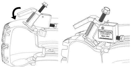
5.3. Using a 3/4" socket or wrench, tighten the clamp bolt on the BeadBuster using a small impact tool or hand wrench. Tighten the clamp bolt until the BeadBuster is vertical, and the body is touching the rim. Make sure the BeadBuster feet are fully inserted. Over-tightening the clamp will cause the tool to lean back and the ram foot to catch on the Bead Retainer of the rim! The Clamp Pad assures that the BeadBuster will not scratch your rims.
