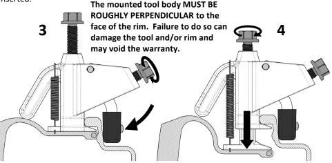
4. Use a 3/4" socket or wrench to run down the Ram Bolt until the Tire Bead has been pushed past the Bead Retainer on rim. Depending on the age of the tire and condition of the rim, the bead may partially return to the seated position. Make sure not to run the Ram Bolt past the point where the flange head contacts the tool body, which may result in stripping out the threads.
