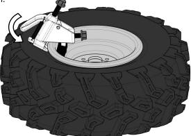
Use a 3/4" socket or wrench to tighten the Clamp Bolt on the BeadBuster using an impact wrench or hand wrench. Tighten the Clamp Bolt until the BeadBuster is vertical, and the body is touching the rim. Make sure the BeadBuster feet are fully inserted.
