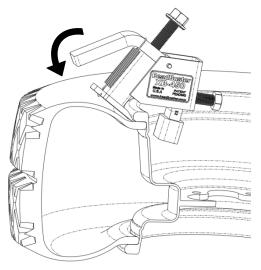
5.3. Using a 3/4" socket or wrench, tighten the clamp bolt on the BeadBuster using a small impact tool or hand wrench. Tighten the clamp bolt until the BeadBuster is vertical, and the body is touching the rim. Make sure the BeadBuster feet are fully inserted. Over-tightening the clamp will cause the tool to lean back and the ram foot to catch on the Bead Retainer of the rim! The Clamp Pad assures that the BeadBuster will not scratch your rims.
