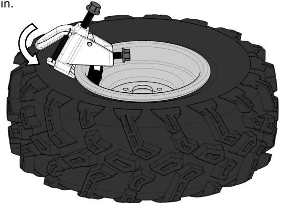
3. Use a 3/4" socket or wrench to tighten the Clamp Bolt on the BeadBuster using an impact wrench or hand wrench. Tighten the Clamp Bolt until the BeadBuster is vertical, and the body is touching the rim. Make sure the BeadBuster feet are fully inserted.
